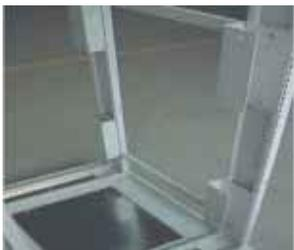
14. This view shows the manner in which the offset brackets are installed opposite each other at the front and back.
