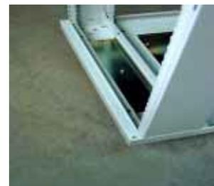
10. Install the plastic shoulder bush hinge in the top/bottom covers on one side and a pair of plastic buttons on the opposite side in the holes provided for them. The plastic buttons are to prevent the door from vibrating during transportation. They need not be used when the rack is in place.
