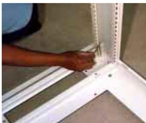
3. Secure the frame to the bottom cover using the nuts and tool provided. Repeat for second frame.
