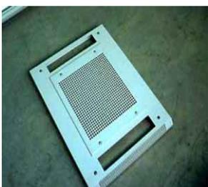
5. Prepare top cover assembly by installing the vented cover plate for the fans and the cable entry cover plates.
